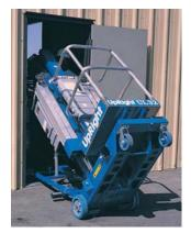
Thanks to the tilt-back system all models will pass through standard single doorways. Large diameter rear wheels on roller bearings move easily over thresholds.
